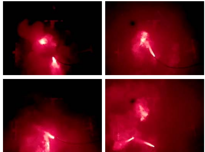
Fig. 4. Video frames from test 3 for an arc flash across a bushing as viewed through an infrared-passing filter.
