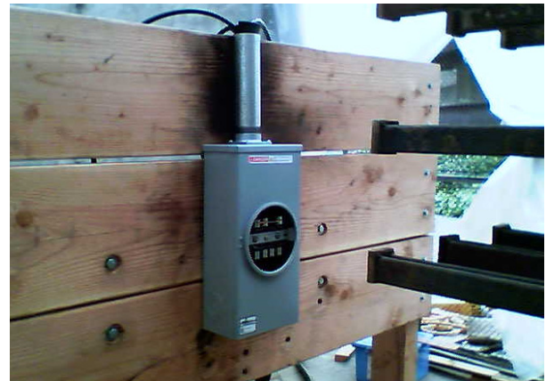
Fig. 1. Self-contained meter test setup
