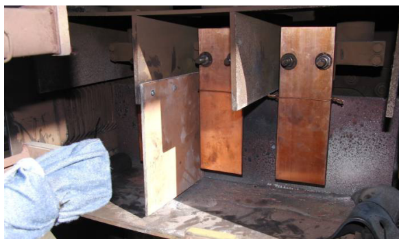
Fig. 28. Test configuration with micarda dividers
