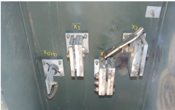
Fig. 11. Vise grip initiated test setup
