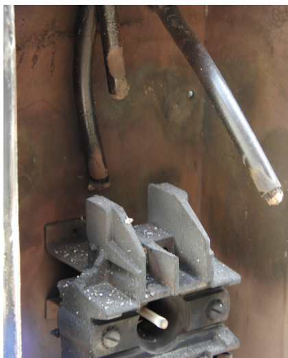
Fig. 3. Meter base after a fault
