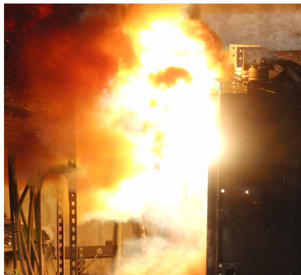
Fig. 40. Typical network protector arc flash
