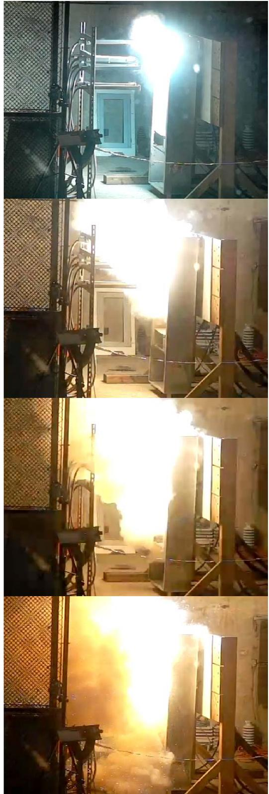
Fig. 30. 250-A power panel for test 232
