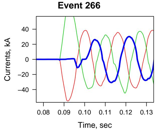
Fig. 46. Current waveforms with a reduced micarda gap
