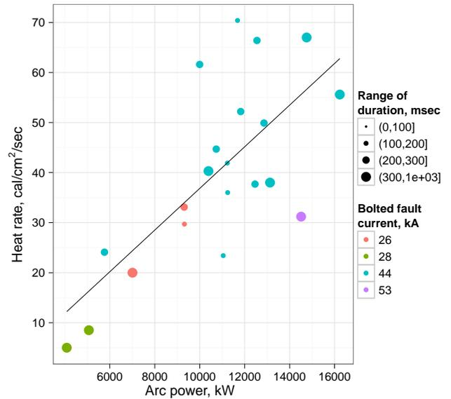
Fig. 50. Arc power vs. incident heat rate
