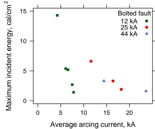
Fig. 25. Maximum incident energy from 50-A and 100-A panels
