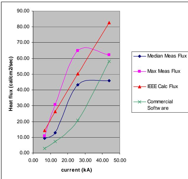
Fig. 7. Measured vs. calculated heat flux for self-contained 480-V three phase meters
