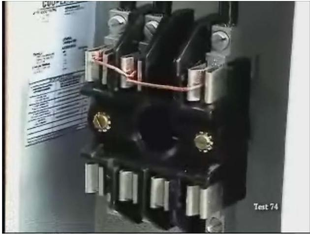
Fig. 3. Shorting wire used to start the fault
