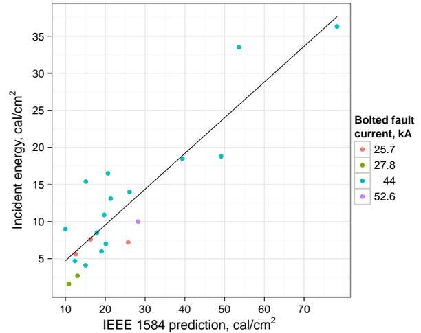
Fig. 53. Measured incident energy vs. calculated (with IEEE 1584 using gap = 2.5" and actual arcing current)
