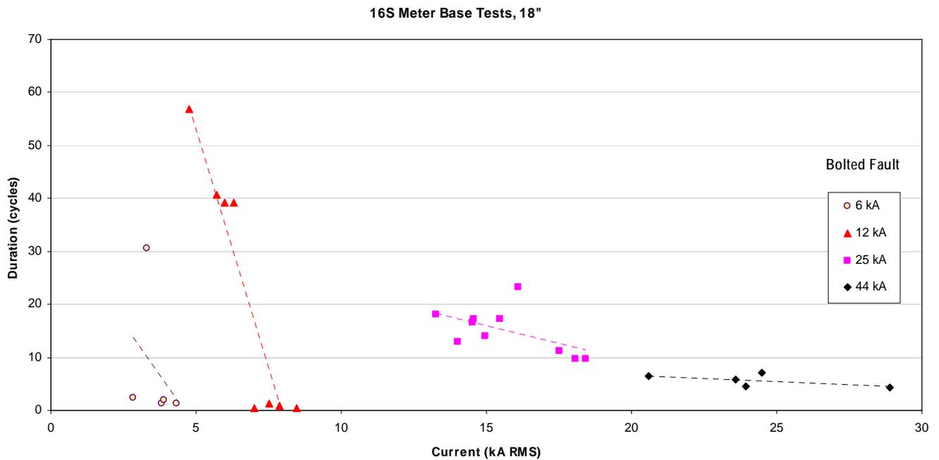
Fig. 5. 480-V meter arc duration vs. arcing fault current
