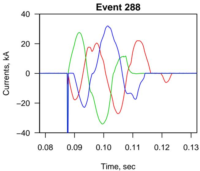
Fig. 16. Current waveforms for a wrench event
