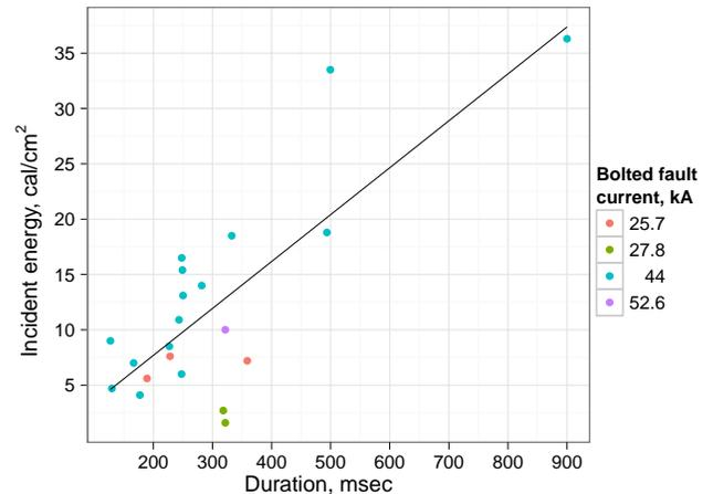
Fig. 47. Incident energy vs. duration
