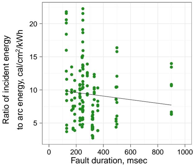
Fig. 49. Energy transfer ratio vs. fault duration
