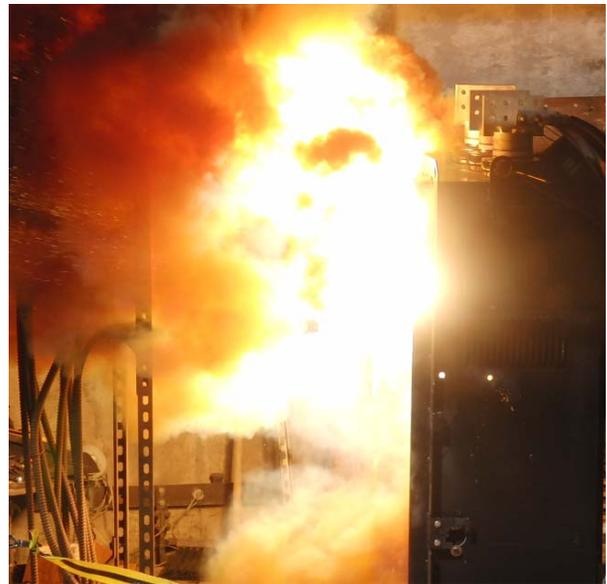
Fig. 57. Typical network protector arc flash
