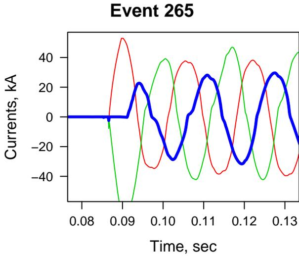
Fig. 44. Current waveforms with micarda spacers
