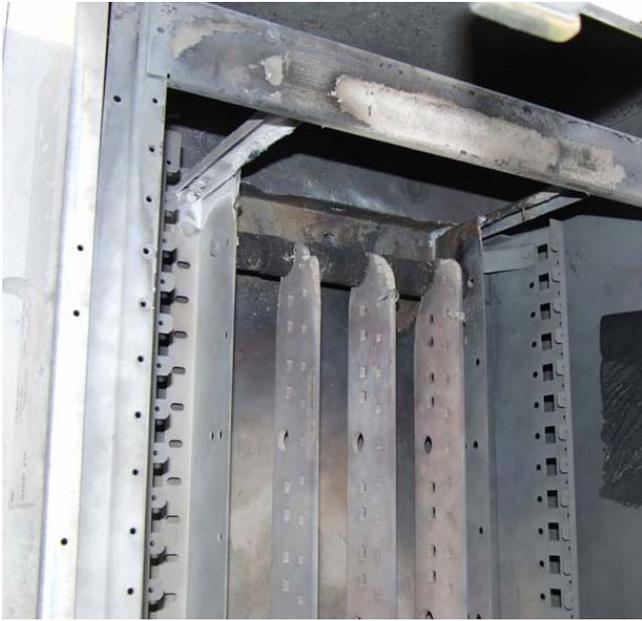
Fig. 28. 250-A power panel after test
