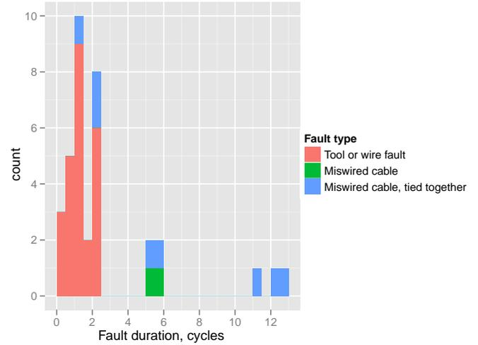
Fig. 22. Fault duration histogram
