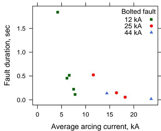
Fig. 26. Fault duration from 50-A and 100-A panels
