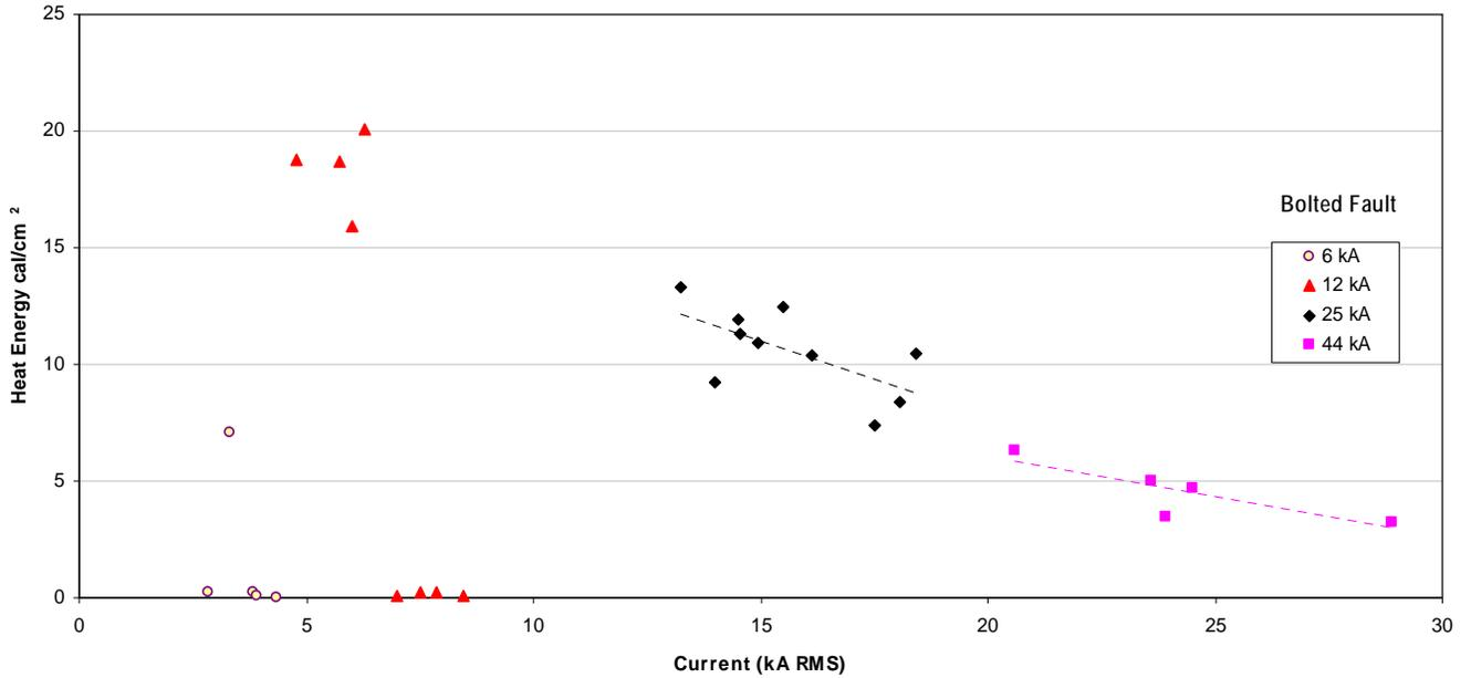
Fig. 6. 480-V meter incident energy vs. arcing fault current
