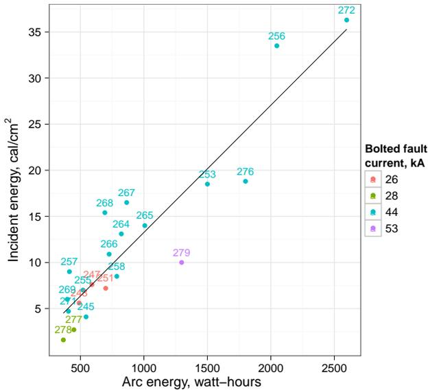
Fig. 48. Comparison of incident energy to arc energy
