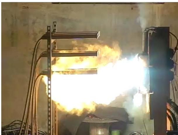
Fig. 56. Typical meter arc flash
