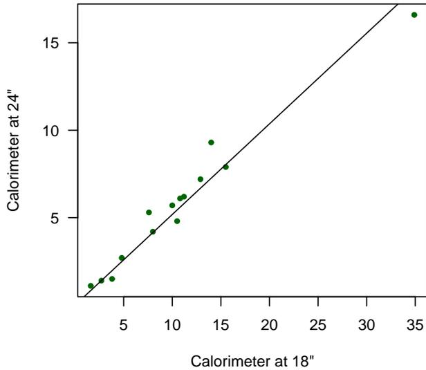
Fig. 52. Incident energy measured at different distances
