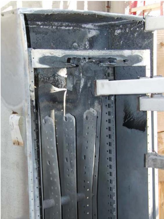
Fig. 31. 250-A panel after test 233
