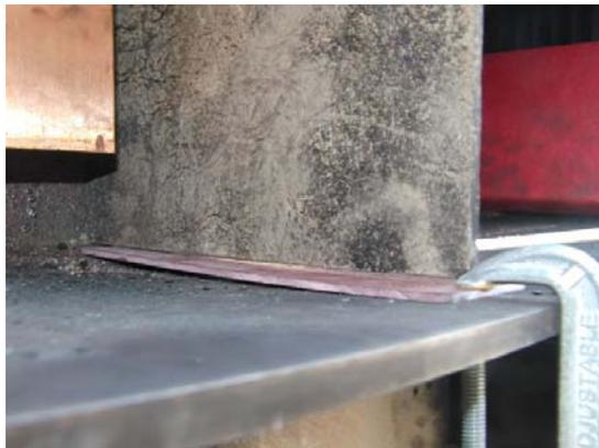
Fig. 45. Reduced micarda spacing
