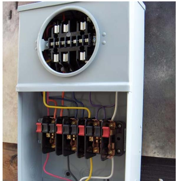
Fig. 8. Transformer rated meter test fixture
