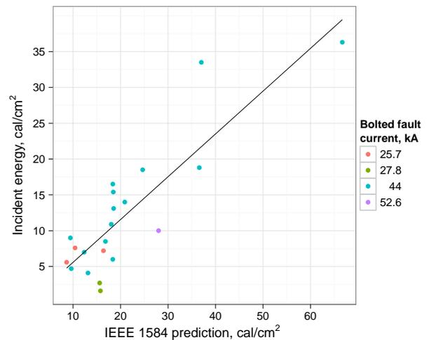
Fig. 54. Measured incident energy vs. calculated (with IEEE 1584 using gap = 1.25" and bolted fault current)
