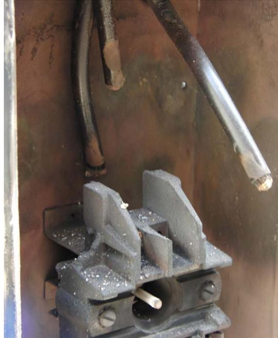
Fig. 4. Meter base after a fault
